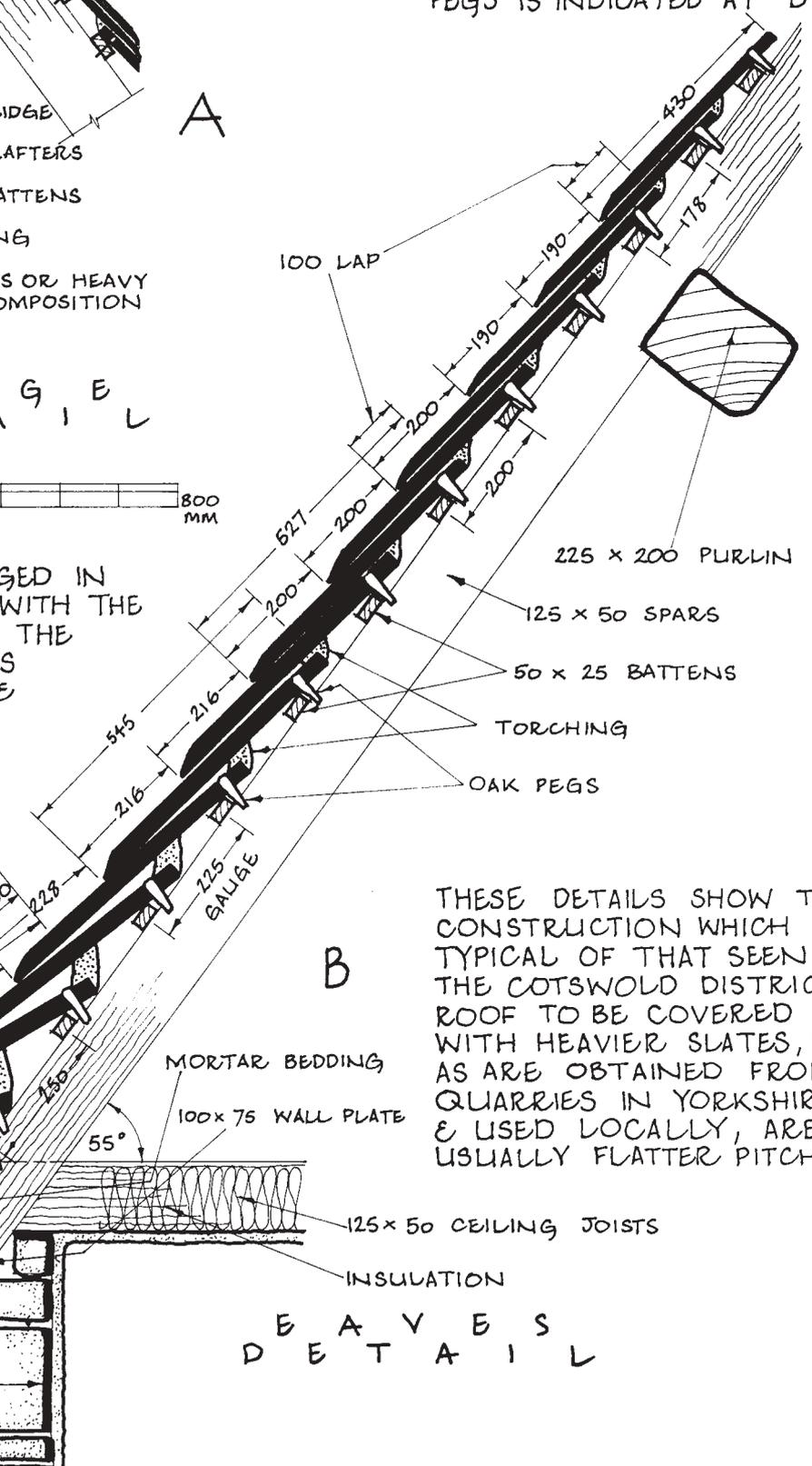
THESE DETAILS SHOW THE CONSTRUCTION WHICH IS TYPICAL OF THAT SEEN IN THE COTSWOLD DISTRICT. ROOF TO BE COVERED WITH HEAVIER SLATES, SUCH AS ARE OBTAINED FROM QUARRIES IN YORKSHIRE & USED LOCALLY, ARE USUALLY FLATTER PITCHED.
