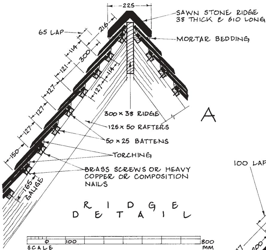
NOTE THE ALTERNATIVE METHODS OF SECURING THE SLATES. THOSE AT "A" ARE SHOWN FIXED BY NAILS OR SCREWS & THE TRADITIONAL METHOD OF HANGING THEM WITH OAK PEGS IS INDICATED AT "B".
