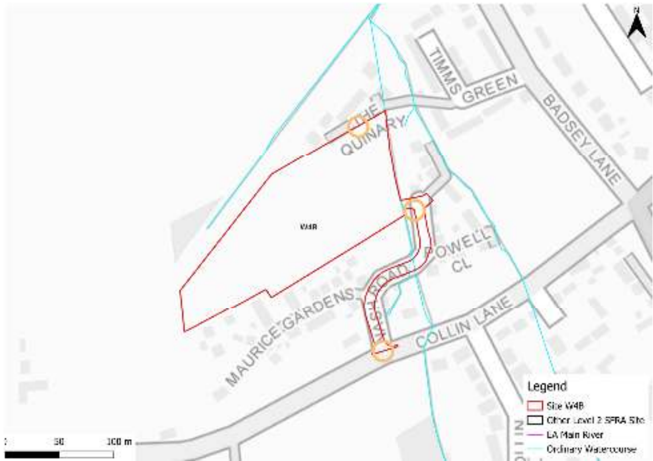
Figure 2-3: Potential access and escape routes
