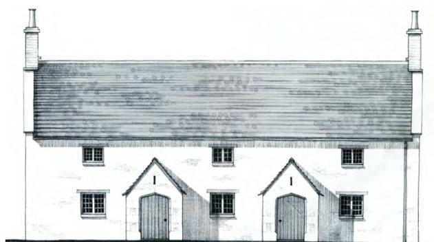
**Figure 24:** A pair of simple 18th - or early 19th century - cottages. Slender brick chimneys are set at the end of coped gables and a 50° 'graded' stone slate roof. Windows are simple iron casements in pegged oak frames, between oak lintels and stone cills. Strong porches of dressed stone with rubble infill have 'sprocket' eaves, mortared verge and plank doors.
