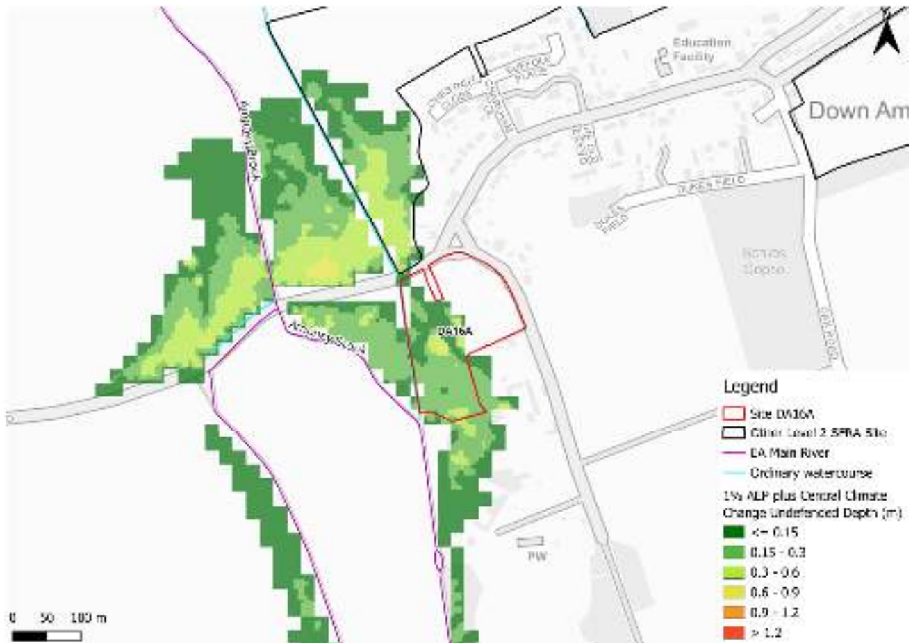
Figure 2-5: Flood depths for the 1% AEP undefended flood event plus central climate change allowance for the 2080s epoch
