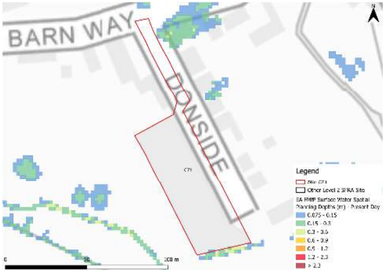
Figure 3-2: Flood Map for Planning - Surface Water Spatial Planning Present Day 0.1% AEP event flood depths (m)
