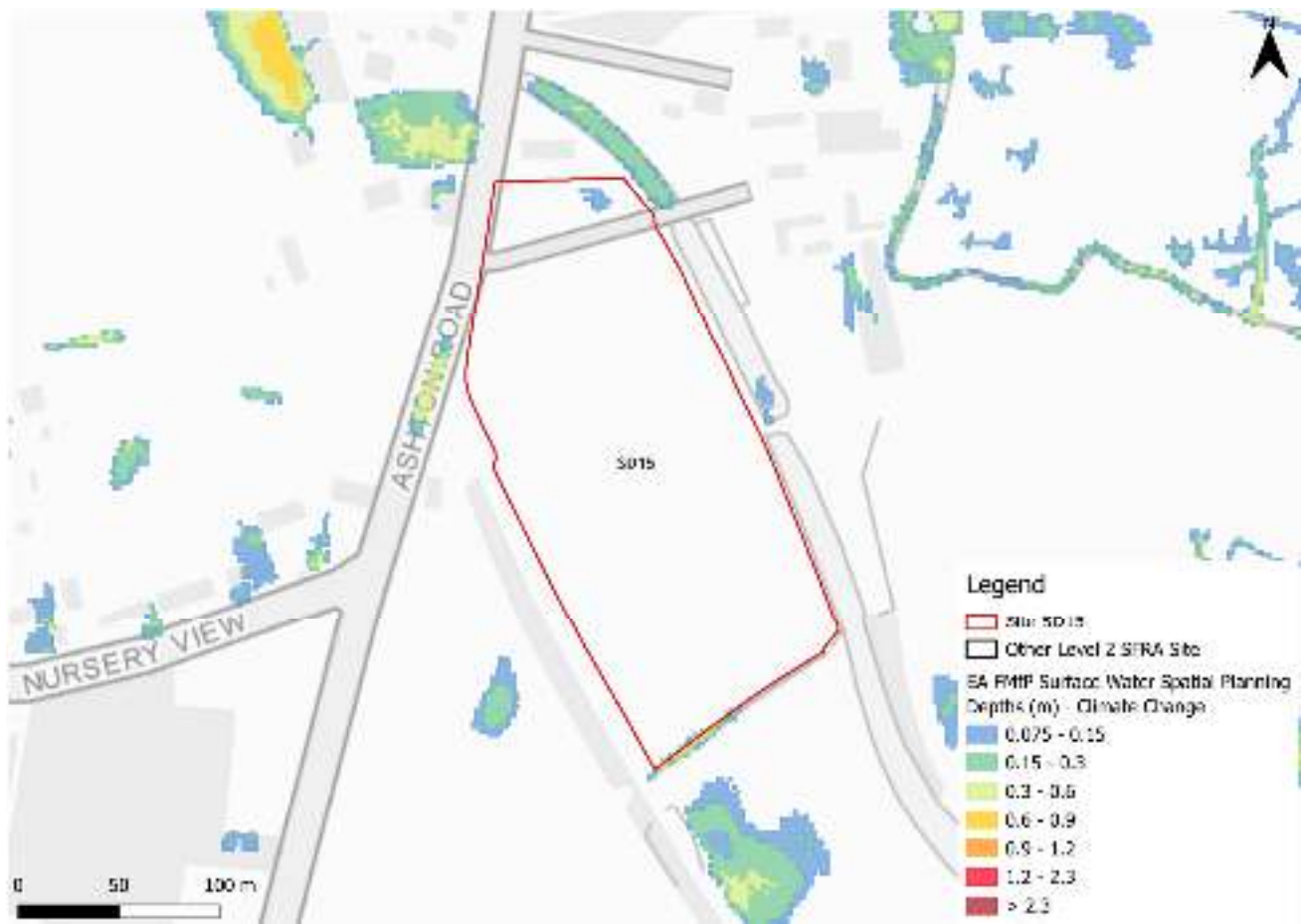
Figure 3-5: Flood Map for Planning - Surface Water Spatial Planning Climate Change 1% AEP event flood depths (m)
