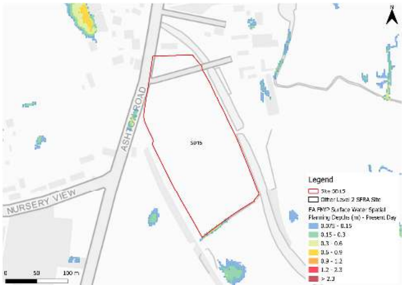
Figure 3-2: Flood Map for Planning - Surface Water Spatial Planning Present Day 1% AEP event flood depths (m)
