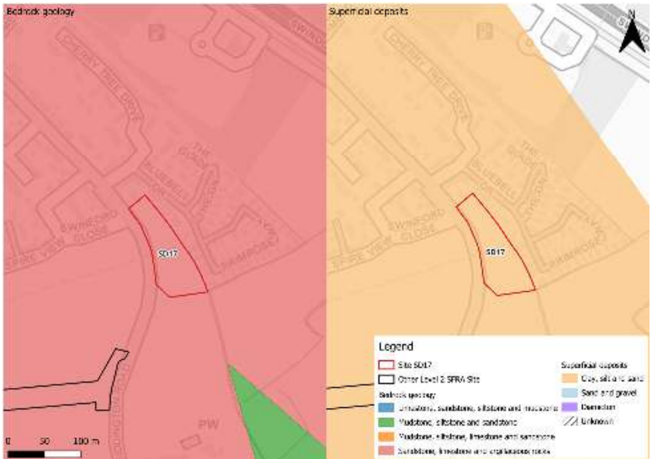
Figure 5-2: BGS Geology - Bedrock and superficial deposits
