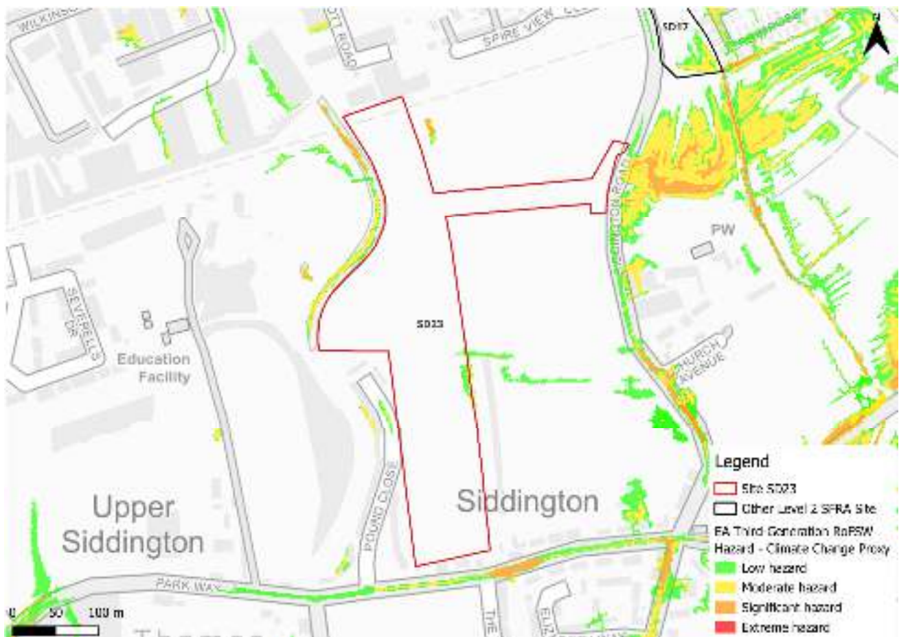
Figure 3-6: Third generation - Risk of Flooding from Surface Water map present day low risk surface water flood hazard as a climate change proxy
